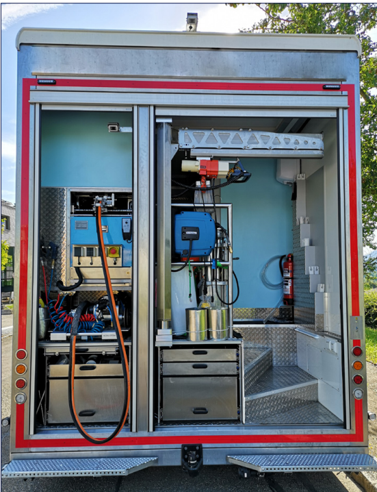
12 - 18 t HYBRID rehabilitation vehicle for KASRO electric working robots for all functions
