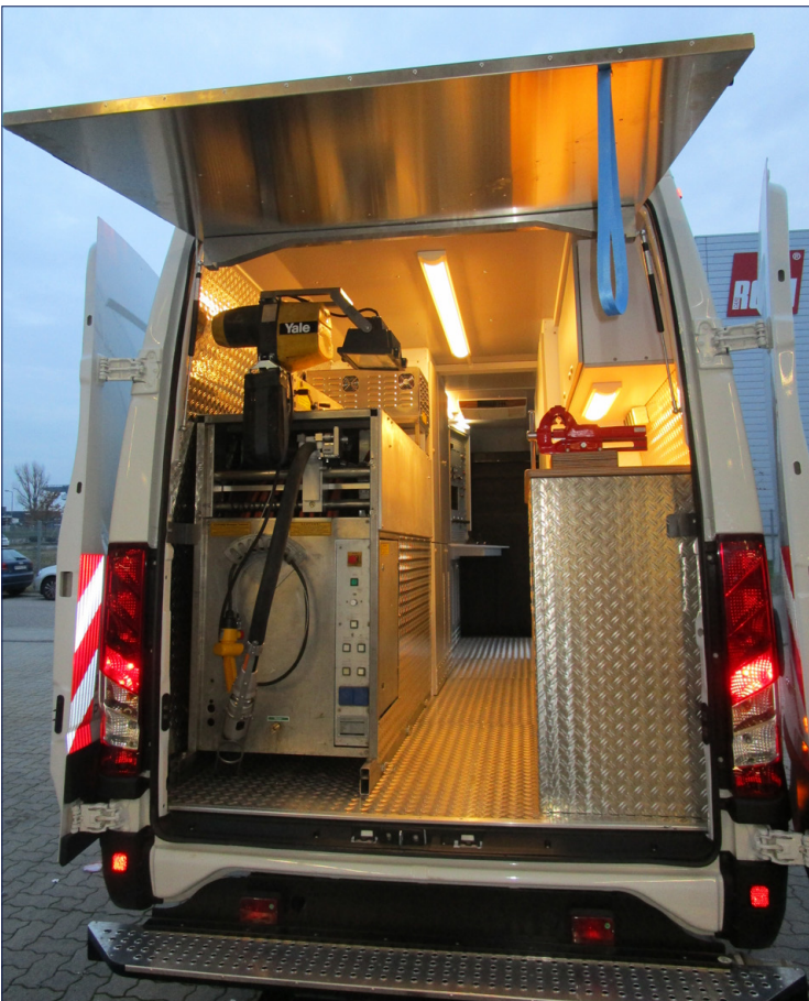
Control unit of the converted KASRO milling vehicle
